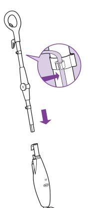
3 Insert the assembled handle piece into the steam mop base. Push the tube base together until you hear a click. (fig. 2)
